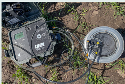
Saturated hydraulic conductivity (shown above) is a measurement of how quickly water enters the soil and is a component of soil moisture dynamics.
